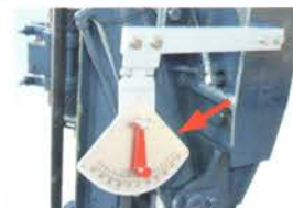
Guide swing angle indicator by pendulum
