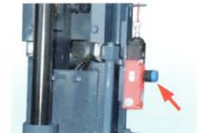
Emergency shut down system
