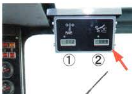
2 dimensional electric angle indicator ① Guide swing angle ② Guide tilt angle
